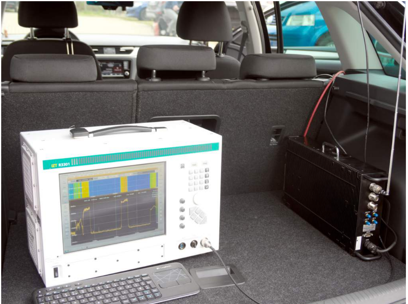
FIGURE 7: RECORDER SETUP WITH IZT R3301 AND IZT R3410
