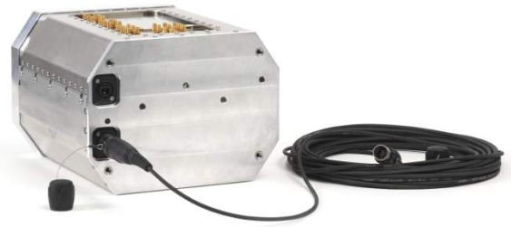
FIGURE 3: IZT R5506 ELECTRONICS WITH HYBRID CABLE.
