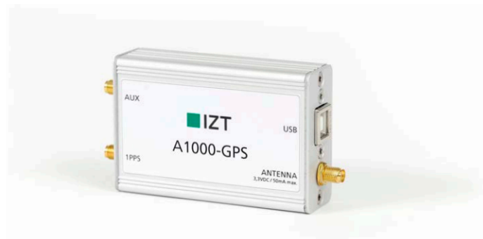
FIGURE 4: EXTERNAL GPS RECEIVER FOR NMEA LOCATION INFORMATION
