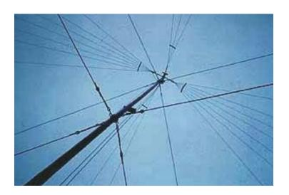
1,5 - 30 MHz Frequency range Impedance 50 ohm **VSWR** < 2,5 (DIAG. 1) Polarization HOR. 1 kW CW Maximum power Radiation diagram DIAG. 2, 3 Height 10 m Lenght of sections 7 X 1,4 m Mass of antenna 67 kg Section diameter 60 mm Mount. time/no. of pers. 30 min./3 Mounting area 25 m Wind velocity 120 km/h Temperature range -40....+70 °C
