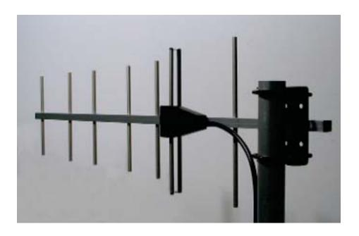
Frequency range 380 - 420 MHz Impedance 50 ohm **VSWR** < 1,6 8,5 dBd Gain Front to Back ratio > 20dB VERT./HOR. Polarization Maximum power 100 W 1.5 m RG-213 + N Connector Width 38 cm 120 cm Length Mass of antenna 2,5 kg
