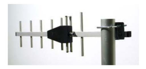
Frequency range 810 - 910 Mhz Impedance 50 ohm **VSWR** < 1,6 8,5 dBd Gain > 20dB Front to Back ratio VERT./HOR. Polarization Maximum power 100 W Connector N female Width 18 cm 64 cm Length Mass of antenna 1 kg
