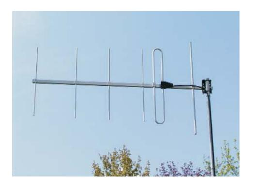
146 - 176 Mhz Frequency range Impedance 50 ohm **VSWR** < 2 8 dBd Gain Front to Back ratio > 14 dB Polarization VERT./HOR. Maximum power 100 W 1.5 m RG-213 + N Connector 100 cm Width Length 180 cm Mass of antenna 5 kg
