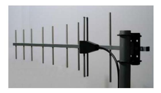
Frequency range 380 - 420 Mhz Impedance 50 ohm VSWR < 1.6 Gain 10 dBd Front to Back ratio > 20dB VERT./HOR. Polarization Maximum power 200 W 1.5 m RG-213 + N Connector Width 38 cm Length 150 cm Mass of antenna 3.0 kg
