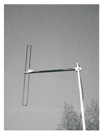
Frequency range 68 - 88 Mhz Impedance 50 ohm VSWR < 1,8 Gain 0 - 2 dBd VERT. Polarization 100 W Maximum power Connector Ν 170 cm Height Lenght 100 cm 2,5 kg Mass of antenna
