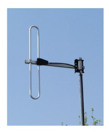
146 - 176 MHz Frequency range 50 ohm Impedance **VSWR** < 1.5 Gain 0 - 2 dBd VERT. Polarization 500 W Maximum power Ν Connector 850 mm Height Lenght 560 mm Weight 2.5 kg 160 km/h Wind velocity
