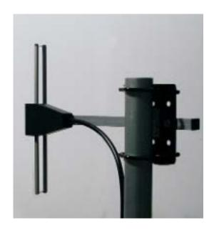
390 - 480 Mhz Frequency range 50 ohm Impedance **VSWR** < 1.8 Gain 0 - 2 dBd Polarization VERT. 100 W Maximum power 1.5 m RG-213/U + Nm Connector Width 30 cm Lenath 31 cm Mass of antenna 2.0 ka
